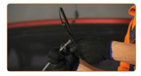
Remove the blade from the wiper arm.
