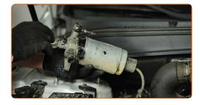
Unscrew the water-in-fuel sensor.
