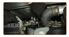
Attach the fuel pressure sensor connector.
