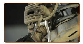
Remove the guide pins from the old brake caliper.
