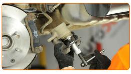
20 Install the brake caliper and fix it.
