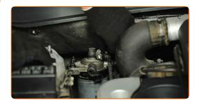
19 Attach the fuel pressure sensor connector.
