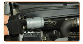
Screw in the water-in-fuel sensor.
