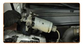
Unscrew the water-in-fuel sensor.
