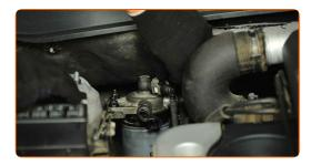
Attach the fuel pressure sensor connector.
