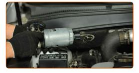
Screw in the water-in-fuel sensor.
