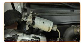
Unscrew the water-in-fuel sensor.
