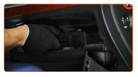
Remove the cabin filter. Use a flat screwdriver.
