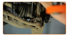
Use a combination spanner #14. Use a drive socket #14. Use a torque wrench. Tighten it to 50 Nm torque.
