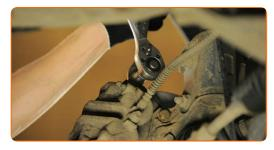
Remove the guide pins from the old brake caliper.
