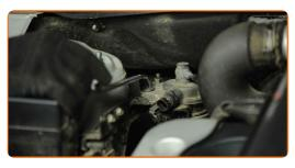
Remove the fuel filter together with its bracket.
