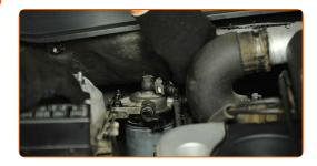
19 Attach the fuel pressure sensor connector.
