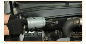
Screw in the water-in-fuel sensor.
