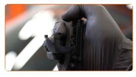
Remove the blade from the wiper arm.
