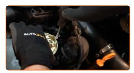
Remove the o-rings. Use a flat screwdriver.
