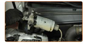
8 Unscrew the water-in-fuel sensor.
