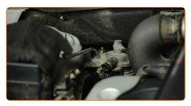
Remove the fuel filter together with its bracket.
