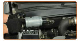
Screw in the water-in-fuel sensor.
