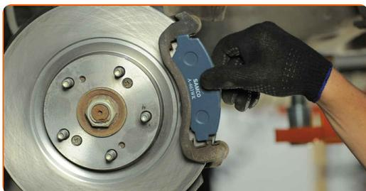
**26** Install the retaining springs of the brake pads.
