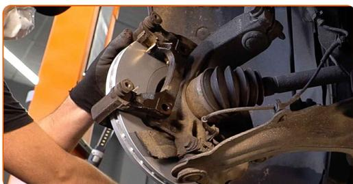
**24** Tighten the brake caliper bracket. Use a drive socket #17. Use a torque wrench. Tighten it to 108 Nm torque.
