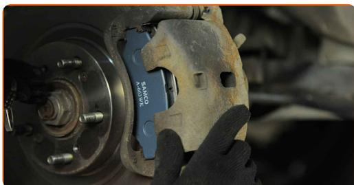
**29.2** Use a drive socket #12. Use a torque wrench. Tighten it to 34 Nm torque.
