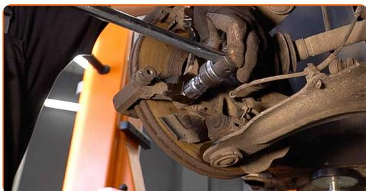
**15** Remove the caliper bracket.
