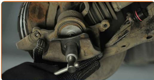
**29.1** Install the brake caliper and fix it.
