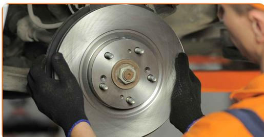
**21** Tighten the brake disc fastening. Use a Phillips screwdriver. Use a torque wrench. Tighten it to 9 Nm torque.
