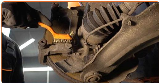
**14** Unscrew the caliper bracket fastening. Use a drive socket #17. Use a ratchet wrench.
