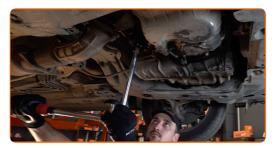
Replacement: engine oil and filter – HONDA Stream II. AUTODOC recommends:
