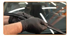
Remove the blade from the wiper arm.
