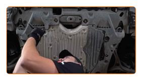
Remove the lower sound insulation. 6
