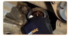
Screw the new filter into its place. Use the 76/14-F socket. Use a torque wrench. Tighten it to 22 nm torque.
