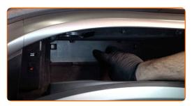
Install the plastic shelf inside the glove box. Close the glove box.
