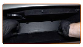
Remove the cabin air filter housing.
