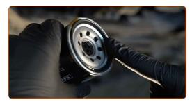
Screw the new filter into its place. Use the 65-14F socket. Use a torque wrench. Tighten it to 18 Nm torque.
