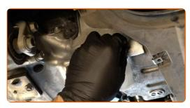
Screw in the new drainage plug and tighten it. Use a drive socket #17. Use a torque wrench. Tighten it to 27 Nm torque.
