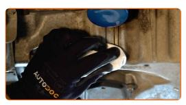
Screw in the new drainage plug and tighten it. Use a drive socket #17. Use a torque wrench. Tighten it to 38 nm torque.
