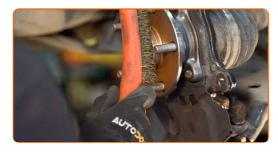
48 Install the brake disc.
