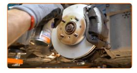
63 Clean the brake disk surface. Use a brake cleaner.
