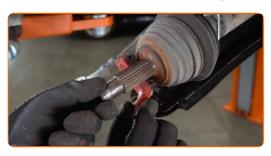
Install the steering knuckle on the CV axle.
