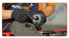
Press the new bearing in the steering knuckle. Use a bush and bearing driver set.
