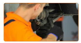
Tighten the fastener connecting the ball joint to the steering knuckle. Use a combination spanner #19. Use a torque wrench. Tighten it to 59 Nm torque.
