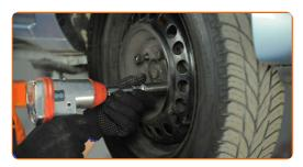
Lower the car and working in a cross order, tighten the wheel bolts. Use wheel impact socket #19. Use a torque wrench. Tighten it to 108 Nm torque.
