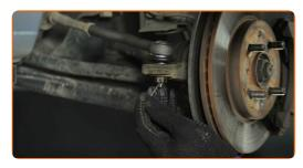
Tighten the tie rod end locknut. Use a combination spanner #19. Use a torque wrench. Tighten it to 44 nm torque. 19
