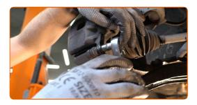
10 Remove the brake caliper.
