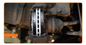
Install the brake caliper and fix it. Use a drive socket #12. Use a torque wrench. Tighten it to 23 Nm torque.
