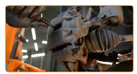
Unscrew the brake caliper fastening. Use a drive socket #12. Use a ratchet wrench.
