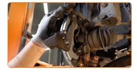
Tighten the brake caliper bracket. Use a drive socket #19. Use a torque wrench. Tighten it to 108 Nm torque.
