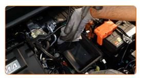
Replacement: air filter – HONDA Jazz III Hatchback (GE\_, GG\_, GP\_, ZA\_). Tip from AUTODOC:
