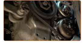
Return the tensioner pulley to its initial position. Use a combination spanner #14.
