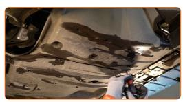
Unscrew and remove the wheel arch cover fasteners. Use a clip removal tool.
