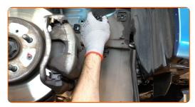
Pull aside the V-ribbed belt tensioner pulley. Use a combination spanner #14.
