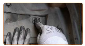
Tighten the fasteners of the oil pan lower cover. Use a Phillips screwdriver.
