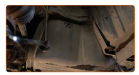
Install and tighten the wheel arch cover fasteners.
