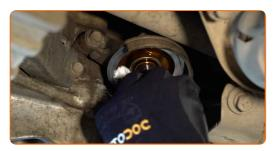
Screw the new filter into its place. Use the 76/14-F socket. Use a torque wrench. Tighten it to 22 nm torque.
