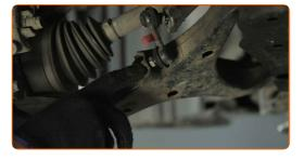
7 Unscrew the fastener connecting the stabilizer link to the stabilizer bar. Use a combination spanner #14 (2 pieces).
