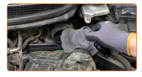
10 Install the air filter cover. Fasten it.
