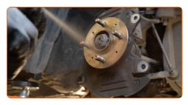
19 Install the brake disc.
