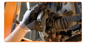
Tighten the brake caliper bracket. Use a drive socket #19. Use a torque wrench. Tighten it to 108 Nm torque.
