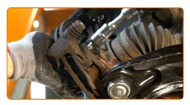
Remove the caliper bracket.
