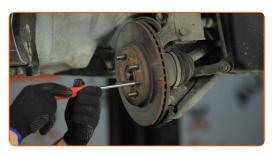
16 Remove the brake disc.
