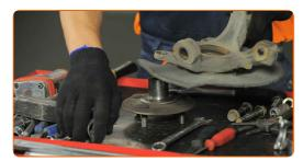
Remove the wheel hub bearing retaining ring. Use round-nose pliers. Use a flat screwdriver.
