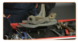
Remove the wheel hub from the steering knuckle. Use a bush and bearing driver set. Use a hammer.
