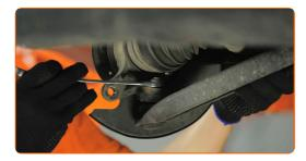
Disconnect the lower arm from the steering knuckle. Use a crowbar. Use a rubber mallet.
