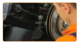
Tighten the fastening nut connecting the tie rod end to the steering knuckle. Use a drive socket #17. Use a torque wrench. Tighten it to 43 nm torque.
