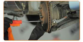
Clean the mounting seats of the caliper and its bracket. Use a wire brush. Use WD-40 spray.
