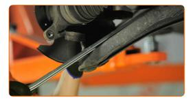
Detach the driveshaft from the steering knuckle.
