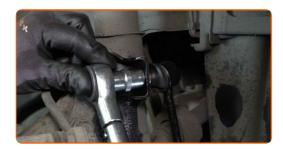
Tighten the fastener connecting the stabilizer link to the stabilizer bar. Use a drive socket #17. Use a torque wrench. Tighten it to 35 Nm torque.
