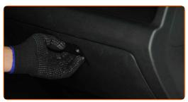
Detach the stopper (strap) from the glove box lid. Use a flat screwdriver.
