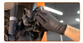
10 Remove the brake caliper.
