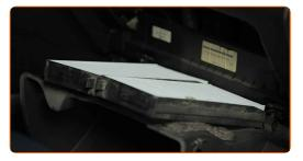
Reinstall the cabin filter housing cover. Make sure you hear a click indicating that it is locked in place.
