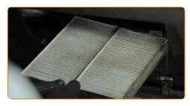
Remove the filter element from the filter housing.
