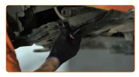
Install the rod fastening to the stabilizer and tighten it. Use a combination spanner #14. Use HEX No.H6. Use a torque wrench. Tighten it to 39 Nm torque.
