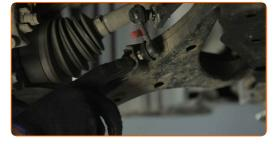
Unscrew the fastener connecting the stabilizer link to the stabilizer bar. Use a combination spanner #14 (2 pieces).
