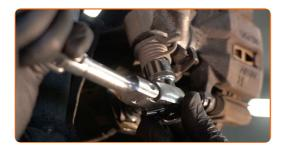
Unscrew the brake caliper fastening. Use a combination spanner #12. Use a combination spanner #17.
