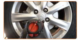
Lower the car and working in a cross order, tighten the wheel bolts. Use wheel impact socket #19. Use a torque wrench. Tighten it to 108 Nm torque.
