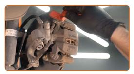
Detach the parking brake cable from the bracket on the brake caliper. Use a drive socket #17. Use a ratchet wrench. Use a crowbar.
