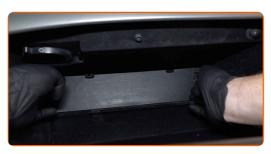
Remove the cabin air filter housing.
