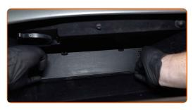
Remove the cabin air filter housing.
