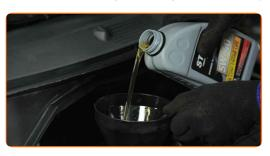
Replacement: engine oil and filter – HONDA Civic IV Hatchback (EC, ED, EE). Tip:
