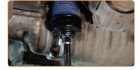
Prepare a container for the old oil filter. Put the old oil filter in the container. 12
