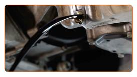
Replacement: engine oil and filter - HONDA Civic III Hatchback (AL, AJ, AG, AH). Tip:
