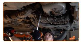
Replacement: engine oil and filter – HONDA Civic III Hatchback (AL, AJ, AG, AH). AUTODOC recommends:
