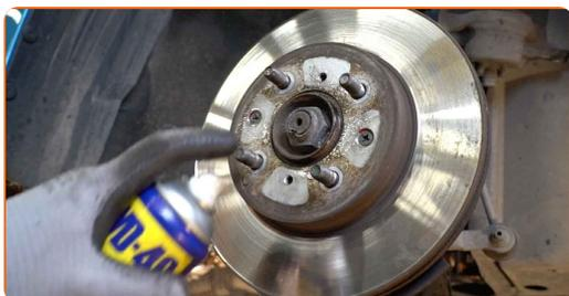
**16** Unscrew the brake disc fastening. Use a Phillips screwdriver. Use an impact screwdriver.
