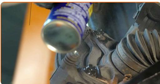
**13** Unscrew the caliper bracket fastening. Use a drive socket #19. Use a tap wrench. Use a ratchet wrench.
