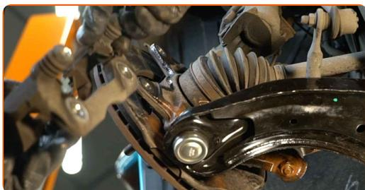
**15** Clean the brake disc fasteners. Use a wire brush. Use WD-40 spray.
