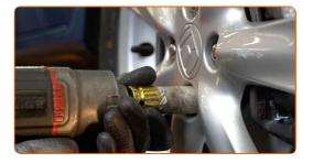
Lower the car and working in a cross order, tighten the wheel bolts. Use wheel impact socket #19. Use a torque wrench. Tighten it to 108 nm torque.
