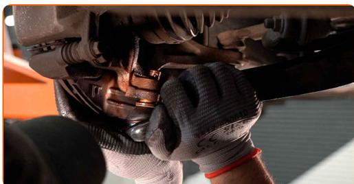
24 Treat the fasteners of the ball joint. Use copper grease.
