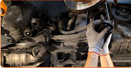
**19** Clean the mounting seats and the thread of the suspension arm. Use a wire brush. Use WD-40 spray.
