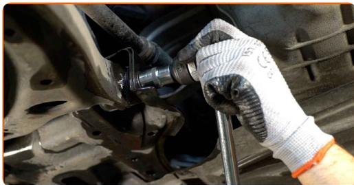
**15** Unscrew the rear fastener connecting the control arm to the subframe. Use a drive socket #19. Use a tap wrench.
