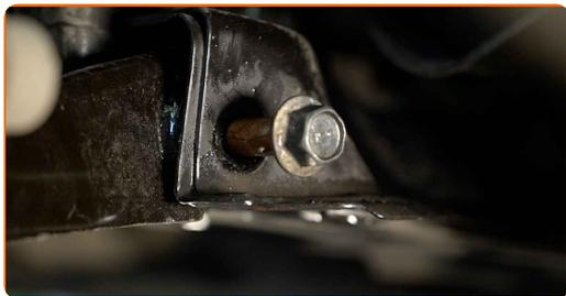
22 Install the rear fastener of the control arm. Use a drive socket #19.
