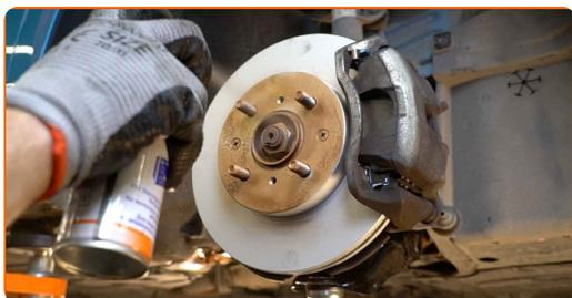
**38** Clean the brake disk surface. Use a brake cleaner.
