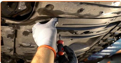
**7** Unscrew and remove the wheel arch cover fasteners. Use a clip removal tool.
