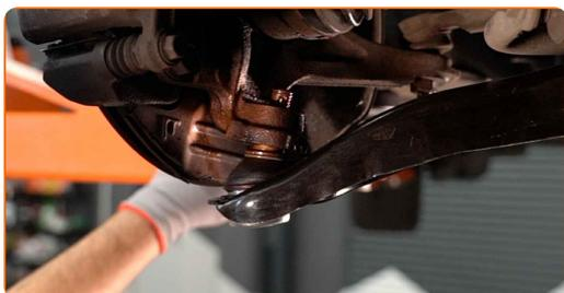
**25** Screw the fasteners of the ball joint. Use a combination spanner #22.
