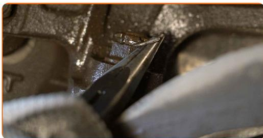
**11** Unscrew the ball joint fastening to the steering knuckle. Use a combination spanner #19.
