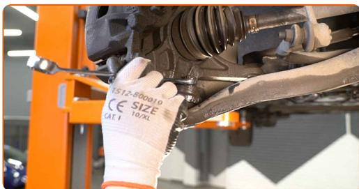
**12** Disconnect the lower arm from the steering knuckle. Use a ball joint puller.
