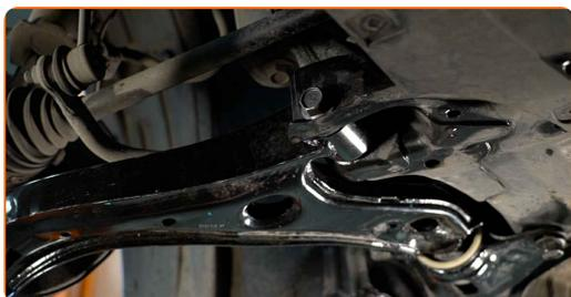
**28** Screw the front arm fastener. Use a drive socket #19.
