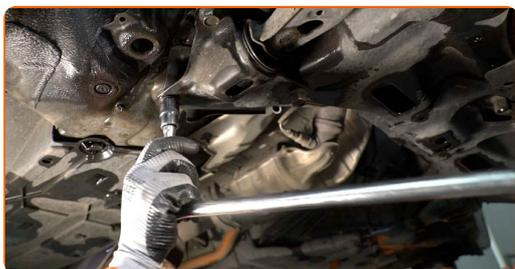
**16** Remove the rear fastener of the control arm. Use a drive socket #19.
