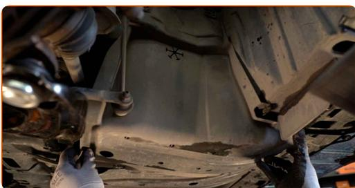
**36** Tighten the fasteners of the oil pan lower cover. Use a Phillips screwdriver.
