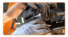
10 Remove the brake caliper.
