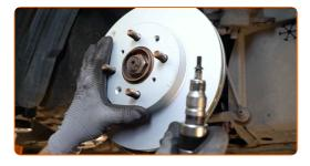
Tighten the brake disc fastening. Use a Phillips screwdriver. Use a torque wrench. Tighten it to 9 Nm torque.
