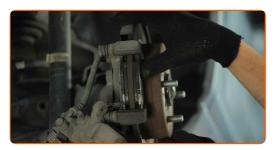
Install the brake caliper and fix it. Use a drive socket #12. Use a torque wrench. Tighten it to 23 Nm torque.
