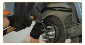
Install the hub bearing protection cap. Use a rubber mallet.
