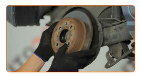
Tighten the brake disc fastening. Use a Phillips screwdriver. Use a torque wrench. Tighten it to 10 Nm torque.
