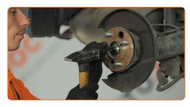
Unscrew the wheel hub axle nut. Use a drive socket #30. Use a ratchet wrench.
