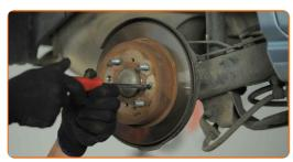
16 Remove the brake disc.
