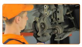
Remove the steering knuckle together with the hub.
