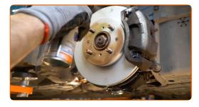
63 Clean the brake disk surface. Use a brake cleaner.
