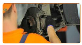
Connect the lower control arm to the steering knuckle. Use a crowbar.
