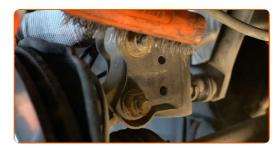
Unscrew the fasteners connecting the suspension strut to the steering knuckle. Use a combination spanner #17. Use a drive socket #17. Use a ratchet wrench.
