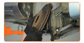
Tighten the brake disc fastening. Use a Phillips screwdriver. Use a torque wrench. Tighten it to 10 Nm torque.
