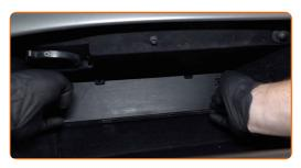
Remove the cabin air filter housing.
